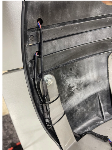
Secure the splitter and wire using zip ties around
