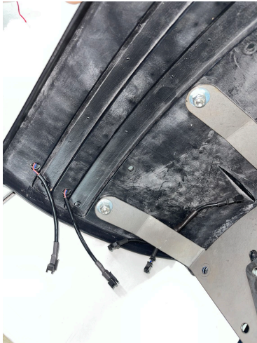
Turn the fender over, use di-electric on all connections to protect it from the elements
