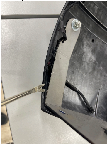
Slide the 1:2 splitter under the lower finger
