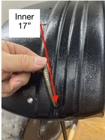
After drilling the appropriate hole, slide the LED tube from the rear and pull forward.
