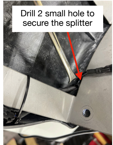
Secure extension and splitter by drilling 2 small holes in the inner plastic under the metal bracket
