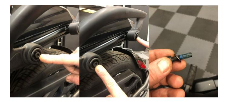
2.-Next take the supplied new bolts with washer and the supplied space and locate the rack with each side arm located over the two bolt locations each side. Place the spacer in the bott location as shown below and move the rack in place. Often it helps to have another person hold the rack while you install all 4 bolts.
