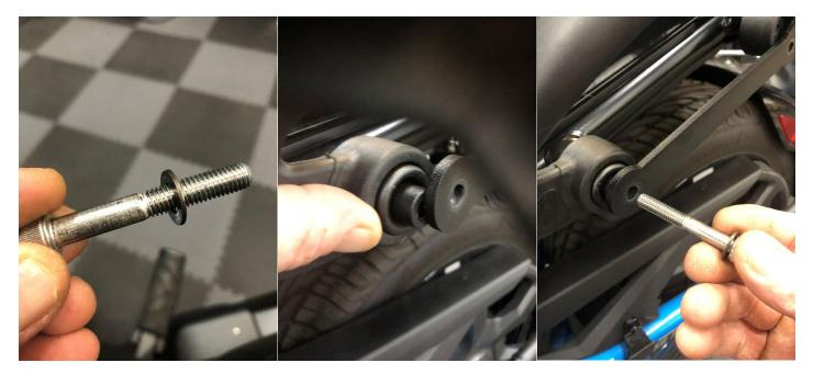
3.- Once all 4 bolts are tightened then take the suppled rubber caps and place over the socket head of each bolt. This completes the installation of your new F3 Rear Carrying Rack. Your Rack can easily carry 20 lbs. of weight.
