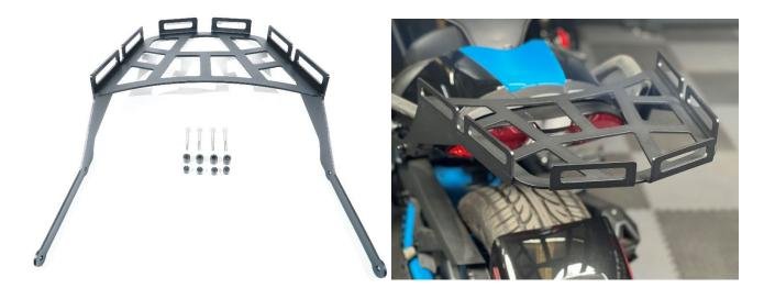
1.- First locate on each side of the two main rear grab bar bolts as shown below. Using a 6mm Allen wrench remove these 2 bolts from each side. When you remove them watch the back side of the grab bar each bolt location to make sure the metal washer does not fall out.
