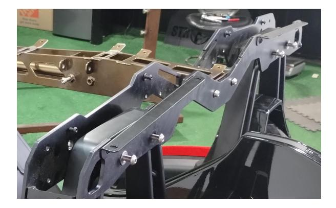
Step 6. **USE TWO PEOPLE. Install center structure to roll hoop mounting plates.** There are four total holes, two in the rear and two in the forward roll hoop mounting plates. Use the provided M8 screws and nuts to fasten the center structure to the roll hoops. Tighten. *You will tighten again as part of the last step*.
