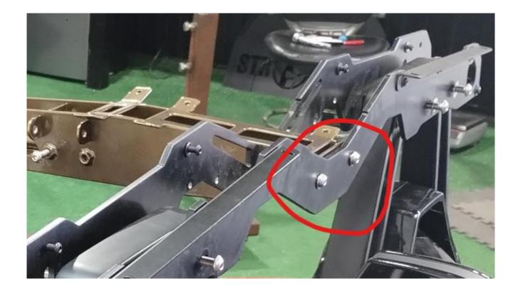
Step 7. **Attach the connecting rods.** Install from top first. <u>Note: **Spacers** and longer</u> <u>screws are used for the *bottom* attachment.</u> Gauge where to pin hole drill the factory cover for the bottom attachment. Next drill the hole to be the diameter of the Heim joint threading.
