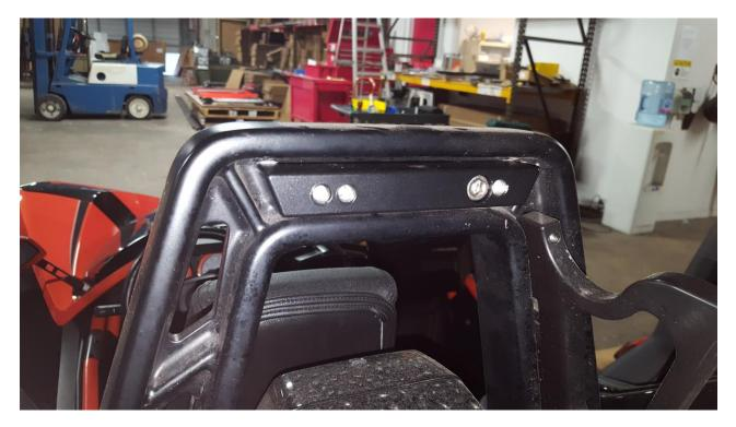
Step 5. **Install roll hoop mounting plates.** *They are not alike, front/rear and up/down orientation*. The screws go into the open holes of the hoop block spacers installed in the previous step.
