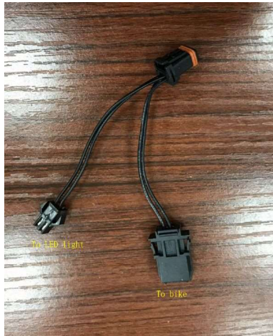
Insert the supplied harness into the OEM harness. This harness will allow you to add other accessories with its male and female end.
