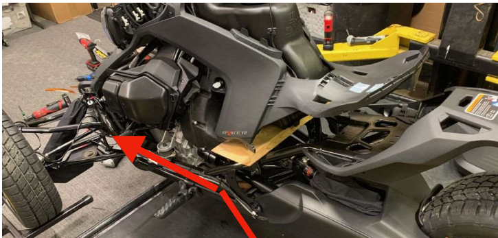
Insert the supplied harness into the OEM harness. This harness will allow you to add other accessories with its male and female end.
