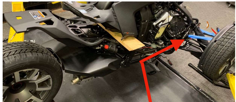
Insert the supplied harness into the OEM harness. This harness will allow you to add other accessories with its male and female end.
