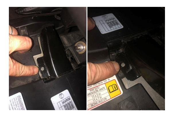
2.- Then take the assembled lift kit and place the main lower mount over the frame so the lower bracket holes line up with the holes above in the frame. The lift kit as the drawing below shows comes with two plastic push pins. Take the two suppled push pins and place them in the two holes and push the pin downward to lock in place.
