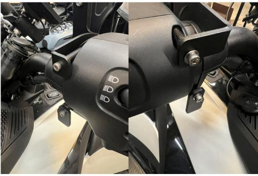
1.- Remove the two 6mm factory Allen screws on the backside of the control module using a 3mm Allen wrench of the side you are mounting you cup older. Left & Right sides determined by rider sitting on your Spyder.
