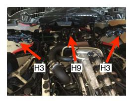
Outboard light(s) uses H3 bulb. Center uses H9. Please note special base used for H3.
