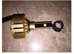
Remove black plastic base. Note the bottom has base lip. This flat base will go into the base of the headlight.
