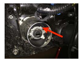
Position the plastic base on the light housing. Make sure it sits flat. There is metal tab on top and bottom and it fits only one way. Once the base sits flat, place the metal clip around the base and rehook on the metal base. Pull the black wire from the ground base of the light (See red arrow above). You will attach this to the black ground on the LED driver. Take your led and line up the side pins and insert into the housing. Once seated flat twist clockwise and lock into place.
