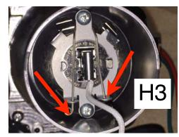
Using a long nose plier, undo the metal clip that holds the factory H3 bulb and remove.
